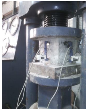
Figure 3: Specimen under Compression
