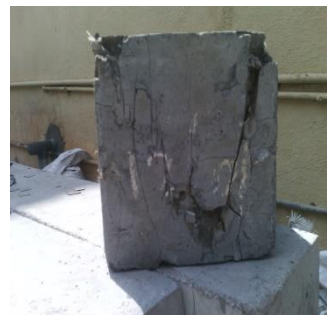
Figure 4: Typical failure mode of specimen
